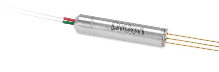
DiCon's **MEMS Optical Attenuator** is based on a micro-electromechanical system (MEMS) chip. The MEMS chip consists of an electrically movable mirror on a silicon support. A voltage applied to the MEMS chip causes the mirror to rotate, which changes the coupling of light between the input and output fibers of the MEMS Optical Attenuator.
